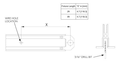
3. HOLDING THE TATE LED<sup>™</sup> UP TO THE GRID WHERE THE HOLE IS DRILLED, PASS THE WIRES THROUGH THE HOLE FROM BELOW THE CEILING. AS THE WIRES ARE PULLED THROUGH, ALIGN THE MOUNTING BRACKETS ON THE TATE LED WITH THE BOTTOM SLOT OF THE GRID AND MAKE SURE THE FIXTURE IS CENTERED ON THE GRID. USING (2) APPROPRIATELY SIZED SCREWS (PROVIDED BY TATE®) FOR THE BOTTOM SLOT, ATTACH THE FIXTURE TO THE GRID.
