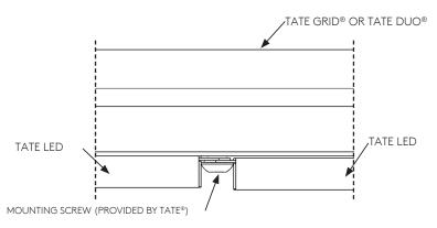
5. WORKING ABOVE THE CEILING PLANE, USE THE PROVIDED METAL JUNCTION BOX WITH MOUNTING PLATE AND PASS THE LOW VOLTAGE WIRES FROM THE TATE LED THROUGH THE SLOT IN THE JUNCTION BOX. SECURE THE JUNCTION BOX WITH MOUNTING PLATE TO THE BACK OF THE GRID USING (2) APPROPRIATELY SIZED SCREWS (PROVIDED BY TATE<sup>®</sup>).
