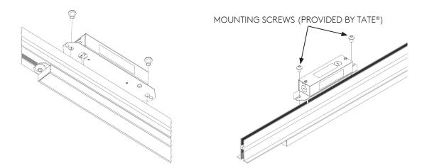
6. VERIFY THE TATE LED FIXTURE IS AGAINST AND CENTERED ON THE GRID. AFTER THE EC HAS ELECTRIFIED THE TATE LED (SEE FOLLOWING PAGE FOR INSTRUCTION), THE CEILING TILES CAN BE PLACED IN THEIR CORRECT POSITION OVER THE TATE LED.
