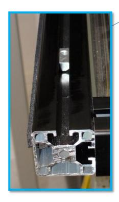
17. Slide piece 3 over the whole of piece 1 and connect using screw 2.
